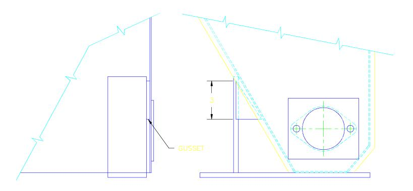
INSTALL GUSSET ON BOTH LEGS BETWEEN END PLATE AND LEG WELD TO LEG AND END PLATE
